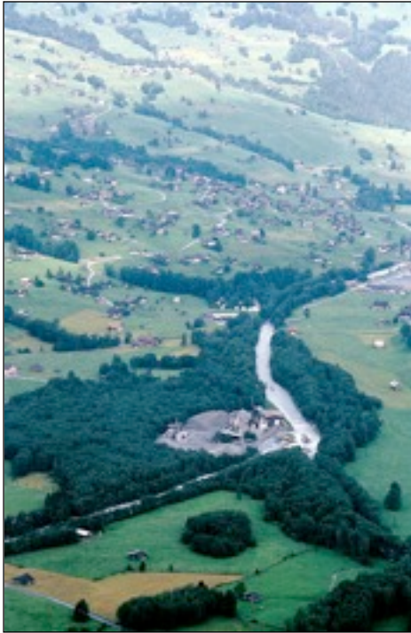
7.128 This gravel mine in the Bernese Oberland causes sediment pollution in the river downstream.
